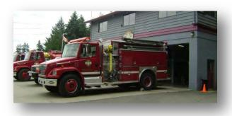
Rapid Attack engine with a compressed air foam system for bush fires. This truck also carries rescue equipment such as auto extrication tools and other rescue equipment. It is equipped with first medical response gear and is the primary response vehicle for this type of incident.
